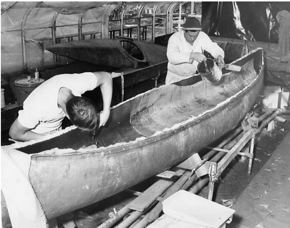
The canoe factory. I am pouring polyester resin into the seventeen-foot canoe mold while my helper, John Ayres, works it into the woven roving with a paint roller. In the background is the deck mold for my C-1. The heating pipes underneath, part of the original nursery propagating house, served to cure the resin more rapidly. Messy work!
